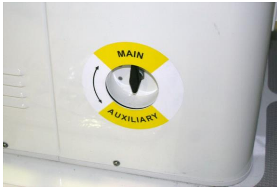
Main/Aux Tank Selector on Engine Box Cover
