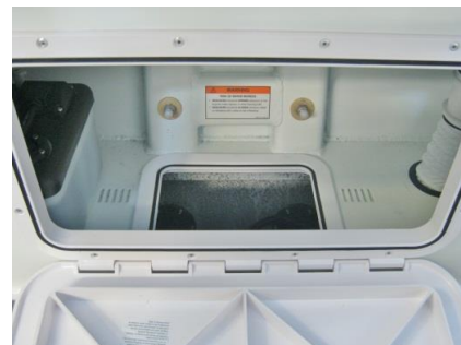
Transom locker and bilge access hatch
