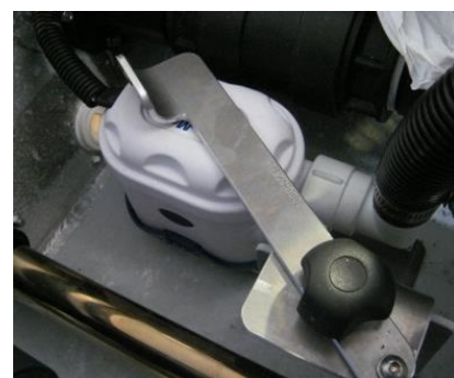
Bilge pump, with locking arm
